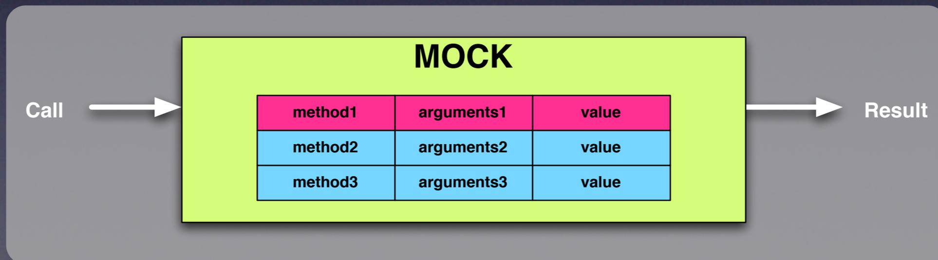
A mock produces a value given calls *after* checking its internal state
